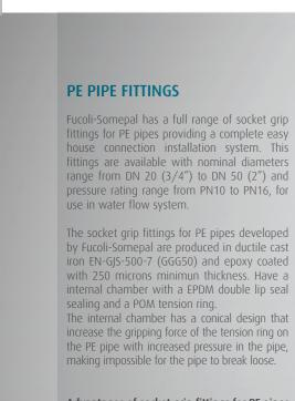
internal chamber with a EPDM double lip seal The internal chamber has a conical design that increase the gripping force of the tension ring on the PE pipe with increased pressure in the pipe,
